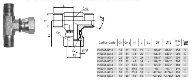
PH1124 CONNETTORE A "T" IN ACCIAIO ZINCATO FILETTO MASCHIO CON LATO FEMMINA GIREVOLE BSPP GALVANIZED STEEL MALE TEE BSPP THREAD AND ONE SIDE WITH SWIVEL FEMALE THREAD
